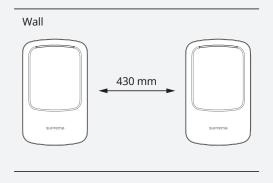
• When using Suprema Mobile Access, install a minimum distance of 1 m between devices to avoid BLE interference.
