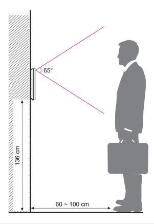
• The optimal height for installing device is 136 cm.
